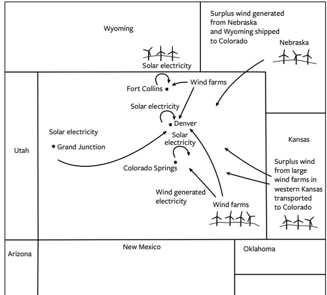
**FIGURE 1.12.** Electricity can be transported from one state or province to another via the electrical grid, a network of high-voltage transmission lines. As illustrated here, surplus electricity from solar and wind energy systems can be transferred to neighboring states, helping to create a steady supply of electricity through rain and shine. Credit: Forrest Chiras.
