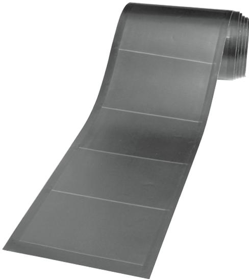
**FIGURE 1.14.** This product, known as PV laminate, is a plastic-coated flexible material that adheres to standing seam metal roofs. It’s best applied to new roof panels *before* they are installed on the building. PV laminate is not as sensitive to high temperatures as conventional silicon-crystal modules used in most solar systems. The company that first developed this product, Uni-Solar is no longer in business, but other companies produce them. Credit: Uni-Solar.
