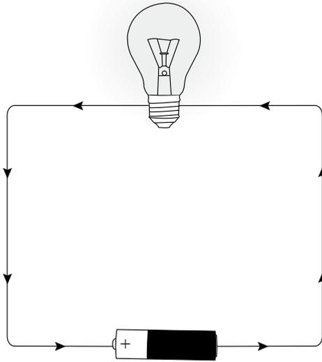
**FIGURE 1.2.** Solar electric systems produce direct current (DC) electricity just like batteries. As shown here, in DC circuits the electrons flow in one direction. The energy the electrons carry is used to power loads like light bulbs, heaters, and electronics. Credit: Forrest Chiras.
