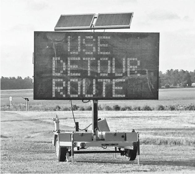
**FIGURE 1.5.** This electronic road sign is powered by a small solar array. Credit: Dan Chiras.
